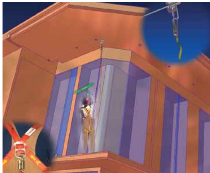
Terminal Anchor With Thaler Energy Absorber (TEA)
